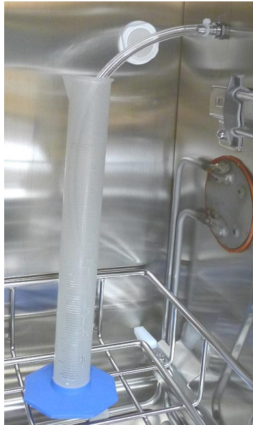
Figure 1: Dosing Pump Test Setup
