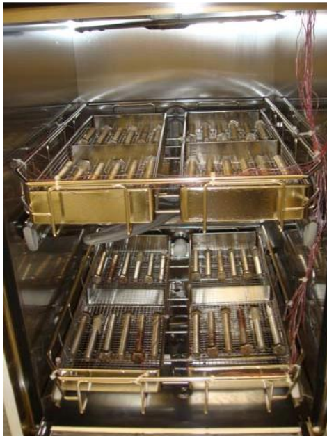
Example of bolt loading in 110 litre unit (double level load carrier shown).
